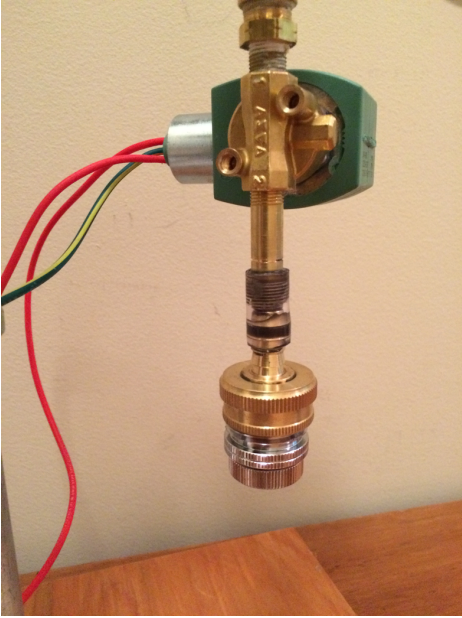
Figure 4-3. Solenoid connection to the macrocarrier holder
