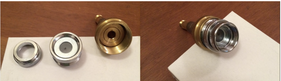
Figure 4-4. Above left, disassembled macrocarrier holder composed of hose fittings; above middle, washers with parafilm and tungsten particles; above right, assembled macrocarrier holder with washers in place
