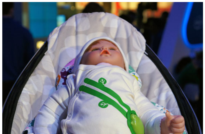
This smart data-collecting onesie for babies monitors heart activity and basic functions. It also activates other baby-gadgets according to the signals detected in the child.
